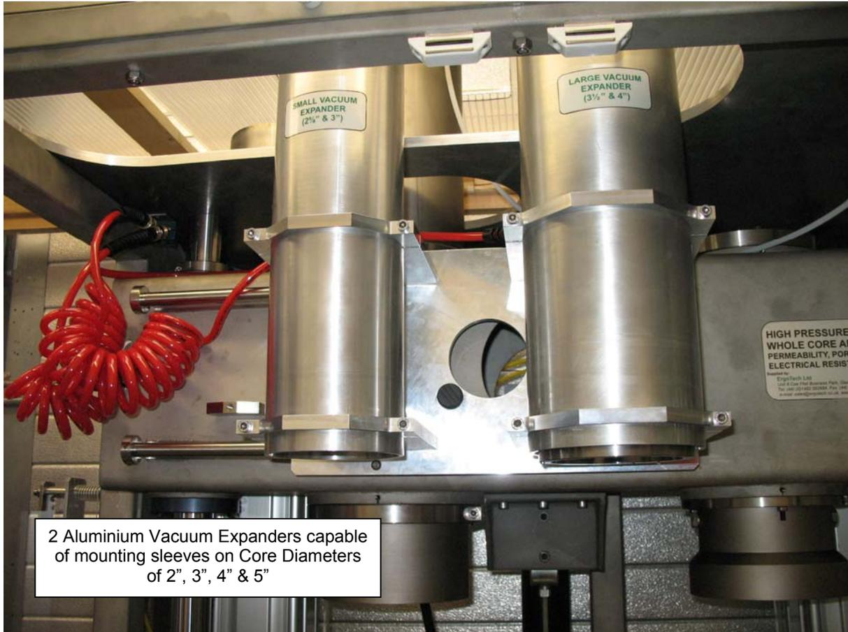
2 Aluminium Vacuum Expanders capable of mounting sleeves on Core Diameters of 2", 3", 4" & 5"
